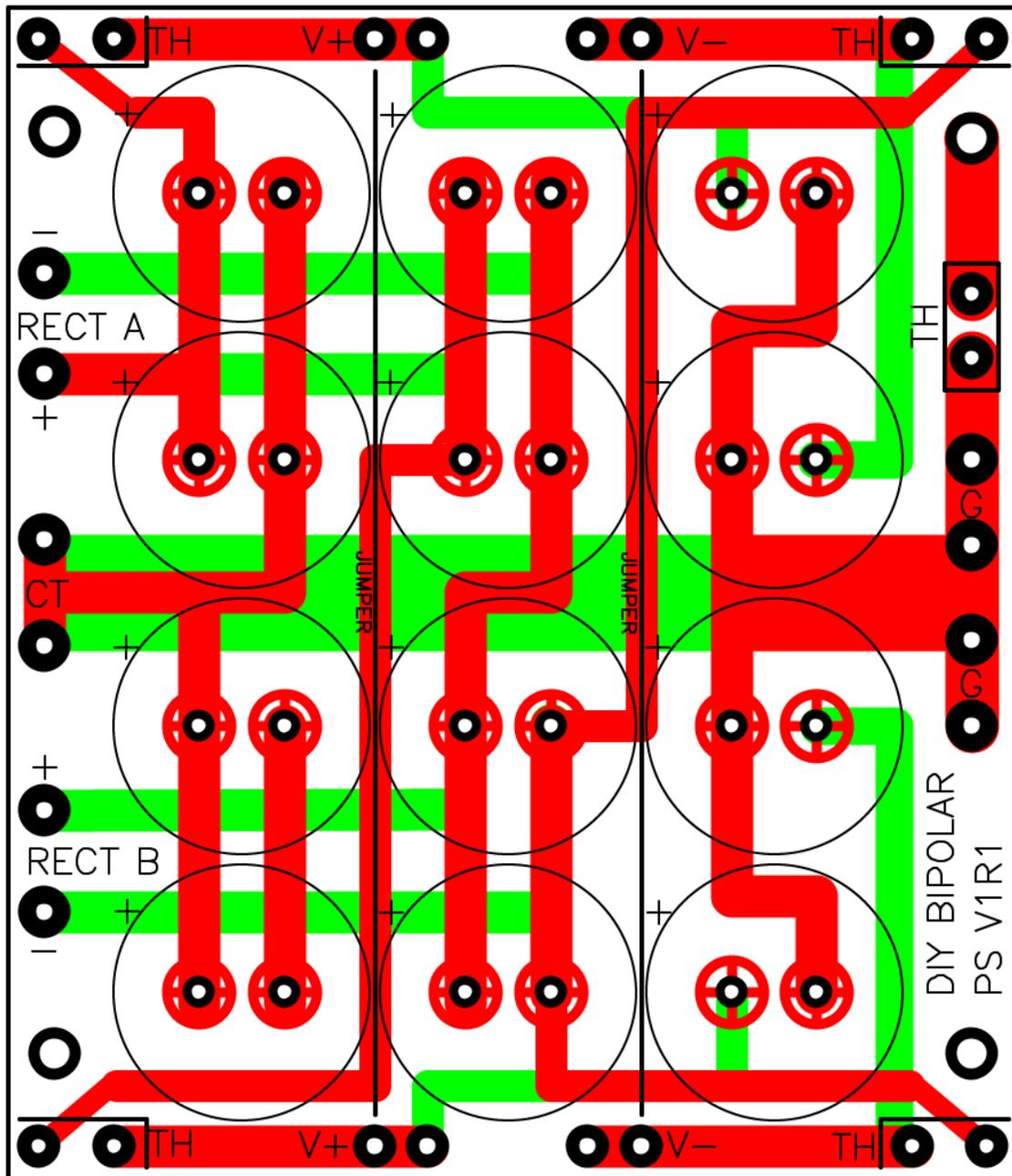
Note also that there are provisions for jumpers between the two channels V+ and V- to allow them to operate in parallel for monoblock operation.
