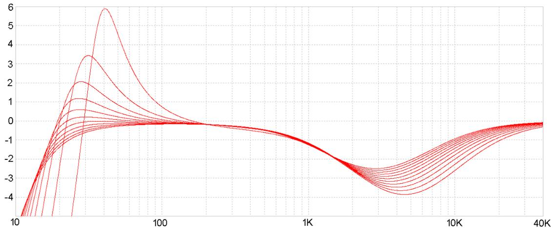
Lower values of R3 give more boost at the low frequency peak and lower values of R5+P1 in series give more attenuation in the midrange dip.
