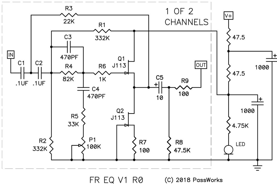
A bass equalization circuit formed by C1-C2 and R1-R3 is followed by the high frequency equalization circuit of C3-C4, R4-R5 and potentiometer P1. Q1 and Q2 form an impedance buffer, and the remaining parts are Fet biasing, output network and power supply filtering.
