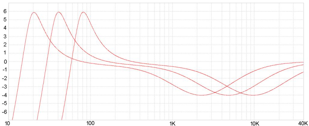
Here are the variations with C1 and C2 at 50 nF, 100 nF and 150 nF at Bass frequencies and C3 and C4 at 0.5 nF, 1 nF and 1.5 nF at the upper frequencies.
