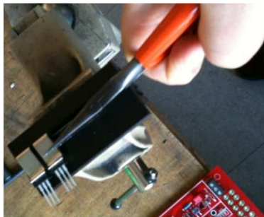
Mounting the power transistors
